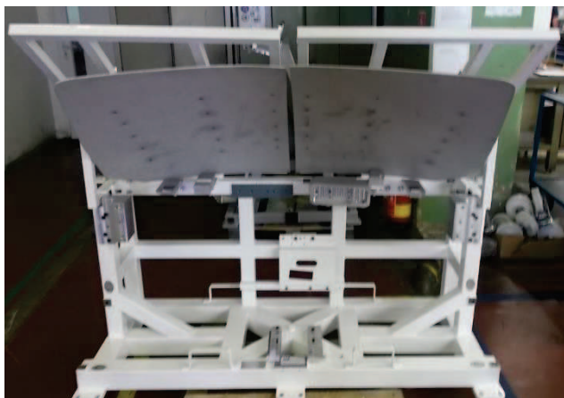
Testing Jig for Bumpers, Tailgate, Door Panel, Instrument Panel
