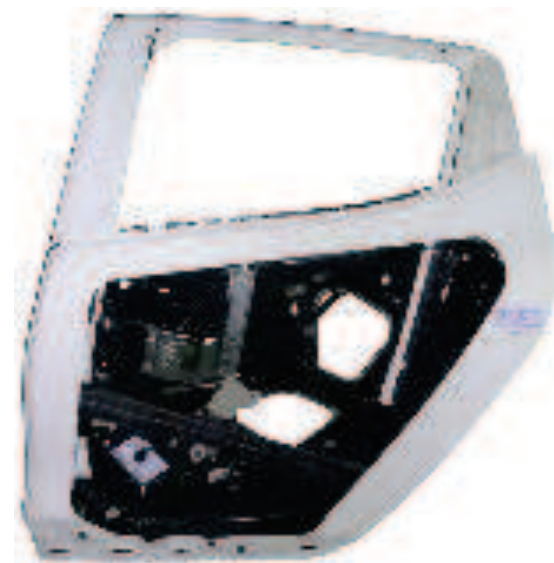
Prototyp Parts in carbon fiber
