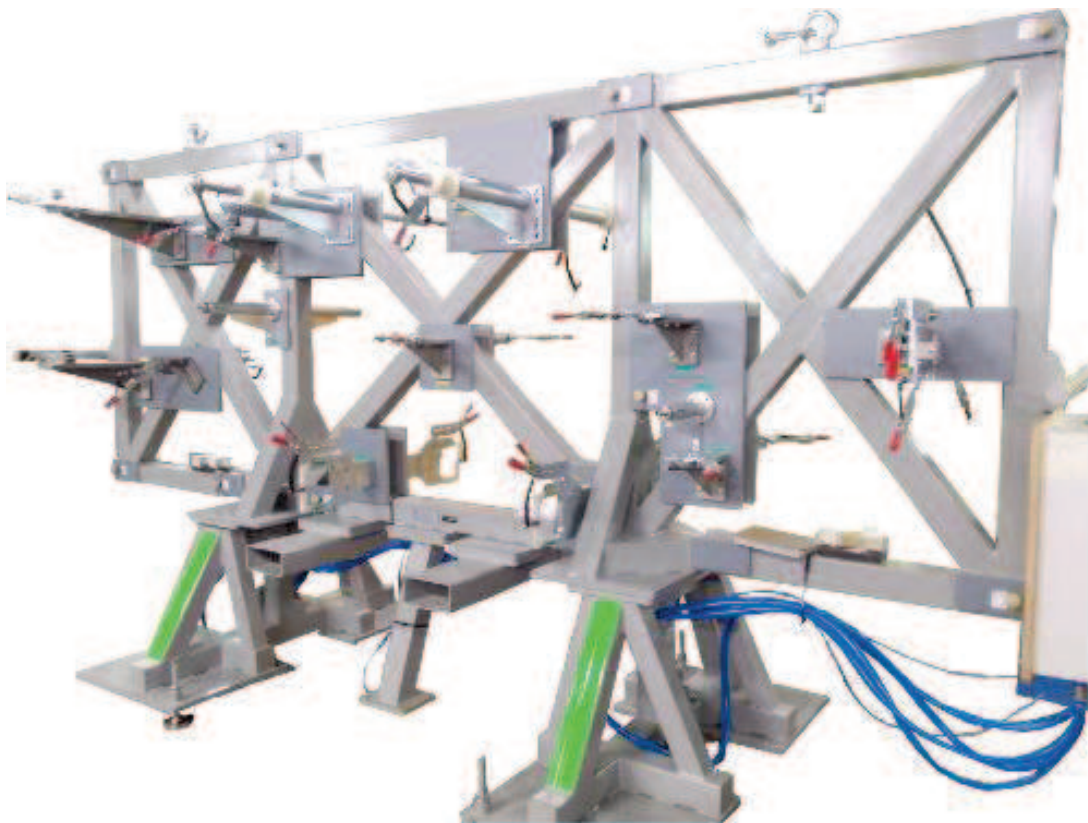
Lateral Body in White Assembly tool
